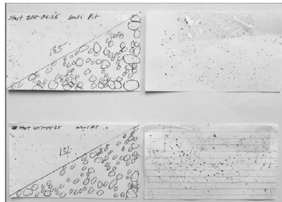
Figure 6. Examples of fly speck cards from a manure pit. Date, location, and number of spots are marked on card fronts.
