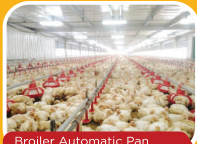
Broiler Automatic Pan Feeding & Drinking System
