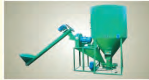
Feed Plant [Feed Mixer & Grinder]
