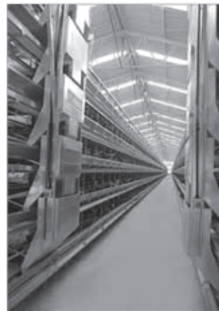
Figure 9. Hopper feeders drop feed directly into the feed trough. Image courtesy Alaso.
