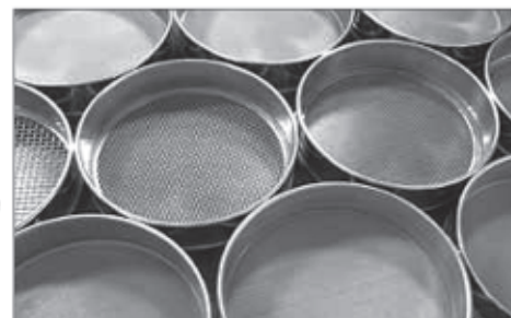
Figure 3. Sieves of varying sizes used to separate a mash feed sample by particle size. Image courtesy Gilson Company, Inc.
