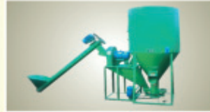
Feed Plant (Feed Mixer & Grinder)
